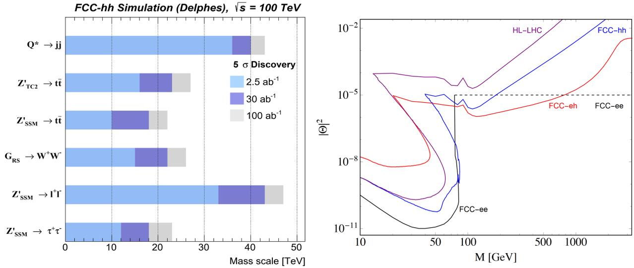
**Figure 5:** Left: FCC-hh mass reach for different s-channel resonances. Right: Summary of heavy sterile neutrino discovery prospects at all FCC facilities. Solid lines show direct searches at FCC-ee (black, in Z decays), FCC-hh (blue in W decays) and FCC-eh (in production from the incoming electron). The dashed line denotes the impact on precision measurements at the FCC-ee, it extends up to more than 60 TeV.
