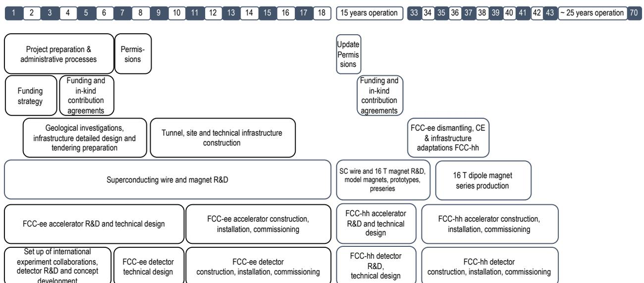
Figure 9: Overview of implementation timeline for the integral FCC program, starting in 2020. Numbers in the top row indicate the year. Physics operation for FCC-ee would start towards the end-2030s; physics operation for FCC-hh would start in the mid-2060s.
