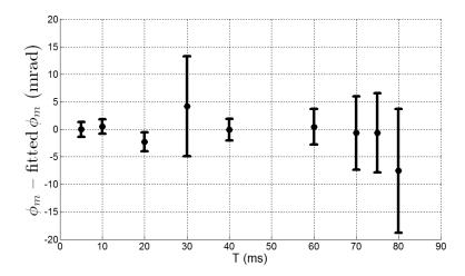
Fig. S9. Speckle Phase Suppression. Anomalous phases measured after subtracting off all other known systematic errors, with the real-time fountain alignment monitor, apodizing filter, and  $N \ge 125$ ; these are the residuals vs T for the data shown in Fig 3C.
