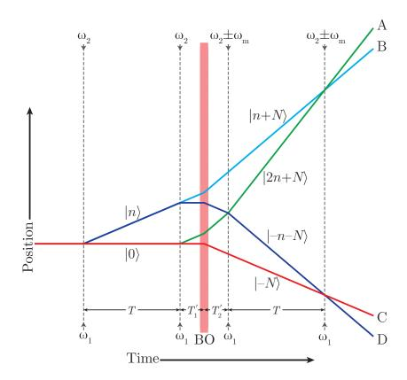
**Fig. 2**. **Simultaneous-Conjugate Atom Interferometers**. The solid lines denote the atoms' trajectories, dashed lines indicate laser pulses with their frequencies indicated.  $|n\rangle$  denotes a momentum eigenstate with momentum  $2n\hbar k$ , where k is the laser wave number. BO; Bloch oscillations. In this figure gravity is neglected.
