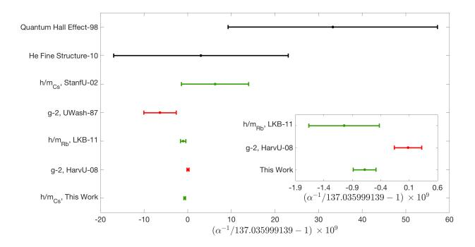
Fig. 1. Precision measurements of the fine structure constant. A comparison of measurements (1, 2, 3, 4, 5, 6, 7, 8). 'Zero' on the plot is the CODATA 2014 recommended value (4). The green points are from photon recoil experiments; the red ones are from electron  $g_e$ -2 measurements.
