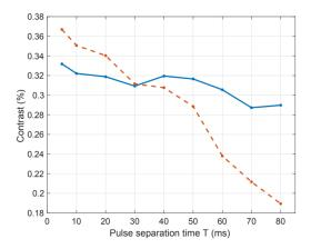
**Figure S2. Contrast vs T.** Contrast in the interferometer as a function of the pulse separation time T is increased, after the addition of the apodizing filter, for N=125. Data with (blue, solid line) and without (red, dashed line) ac-Stark compensation is shown. The integration rate of the experiment is proportional to both the contrast and the pulse separation time.
