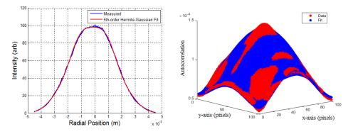
**Fig. S4. Beam profile.** Intensity profile of the apodized beam, measured using the scanning slit beam profiler (left) and the 2-D autocorrelation function of the intensity as determined from a CCD beam profiler. The x and y axes are measured in pixels; 1 pixel corresponds to 6.25μm.
