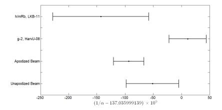
**Fig. S6. Comparing Beam Waists.** Experimental measurements of  $\alpha$ , for two different beam sizes (the unapodized 5.7 mm beam, and the apodized flat-top beam). Also plotted are the LKB-11 and  $g_e$ -2 measurements of  $\alpha$  for reference.
