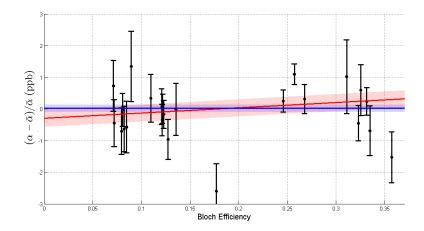
**Fig. S5. Varying Bloch Intensity.** Experimental measurements of  $\alpha$ , as the Bloch efficiency (i.e. intensity) is varied. The blue line is the final reported value of  $\alpha$ , assuming no dependence on Bloch efficiency. The red line assumes a linear dependence; the shaded regions represent 1-sigma error bars.
