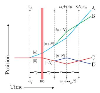
**Fig. S7. Gradiometer Geometry.** The interferometer geometry used to measure the gravity gradient.
