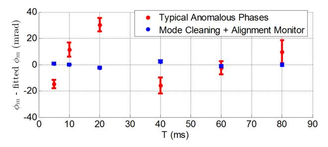
**Fig. S8. Speckle Phase Suppression.** Anomalous phases measured after subtracting off all other known systematic errors, with N = 0. With no effort taken to suppress them, the speckle phases can be as large as 30 mrad (red data). With the real-time fountain monitor and apodizing filter, the speckle phases are kept below 3 mrad.
