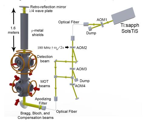
Figure S1. Diagram of the apparatus.
